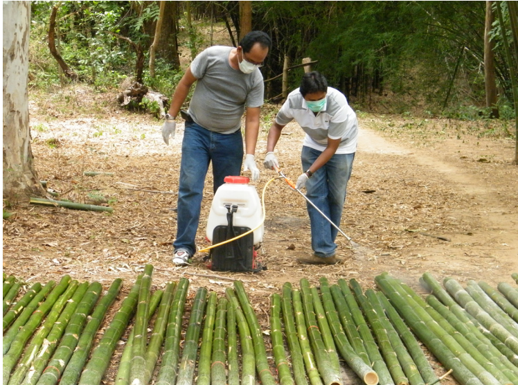
Figure 13 Wood preservative spraying.
